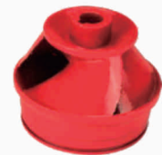
Mixed flow impeller Used for submersible, mixed flow pump with low head and large volume.
